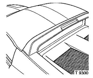
The hardtop is attached to the windscreen frame by means of three bolts and to the rear header rail by means of two quick release fasteners.
